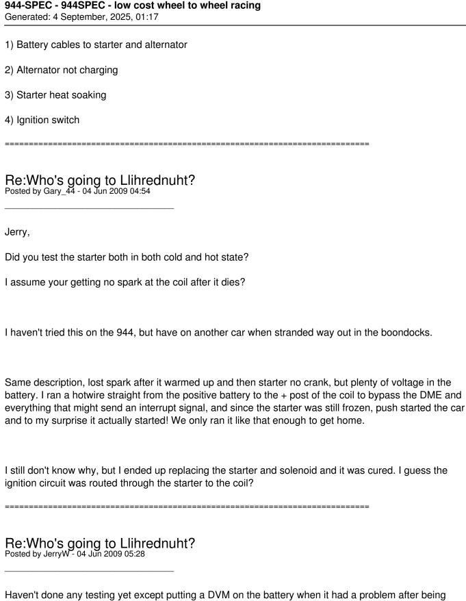
towed in. Strange thing is that adding a jump box allowed it to start. So on Sat after the failure I put a new full size battery in place of the lightweight. Problem happened again on Sunday with the new battery within the day.
