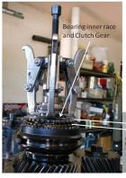
7a-Here is the bearing race/clutch gear and syncro once you pull them off
